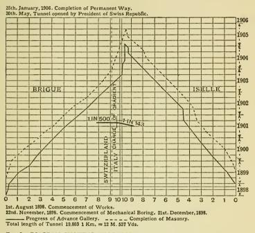
FIG. 8.—DIAGRAM SHOWING PROGRESS OF ADVANCE GALLERY AND COM-PLETION OF MASONRY FOR TUNNEL No. 1.
